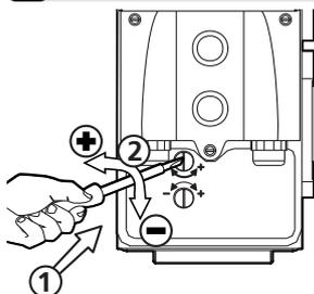
Locate the screw which controls direction of the rotation "UP" and the one which controls direction of the rotation "DOWN" ; direction 1 or direction 2. Arrows located around the hollow shaft indicate also the direction of rotation.
