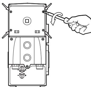
1. Remove the chain cover by unscrewing the 4 screws.
